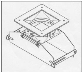
The adjustable V R discharge funnel is used in conjunction with the standard TUC quick release fitting to enable concrete to be poured into very narrow moulds associated with prefabrication work.
